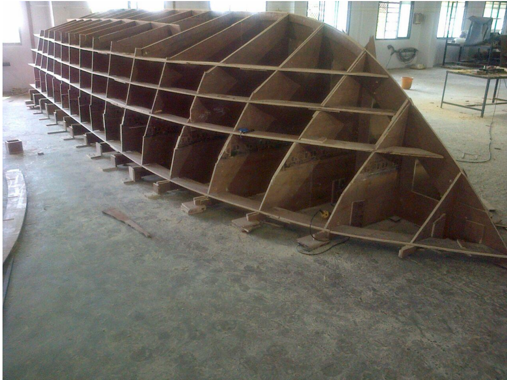
Photo 10: Making of Plug for Survey Motor Boat
